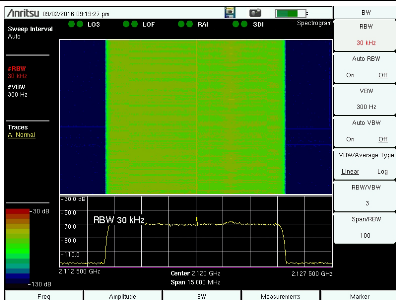
Figure 2-5. CPRI Spectrogram Display
