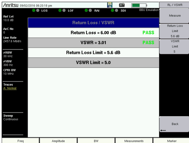
Figure 2-49. Return Loss/VSWR Measurement Results
