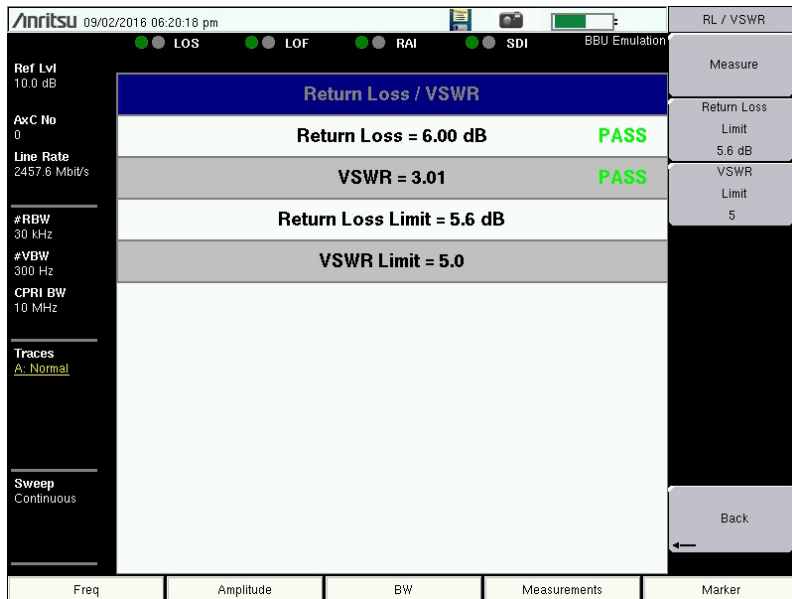
Figure 2-17. Return Loss/VSWR Measurement Results
