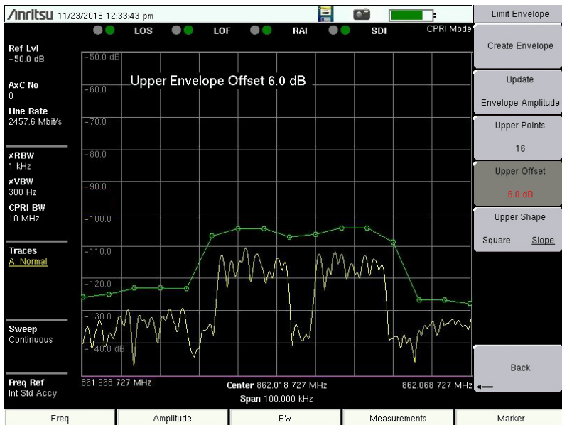
Figure 2-73. Sloped Limit Envelope
